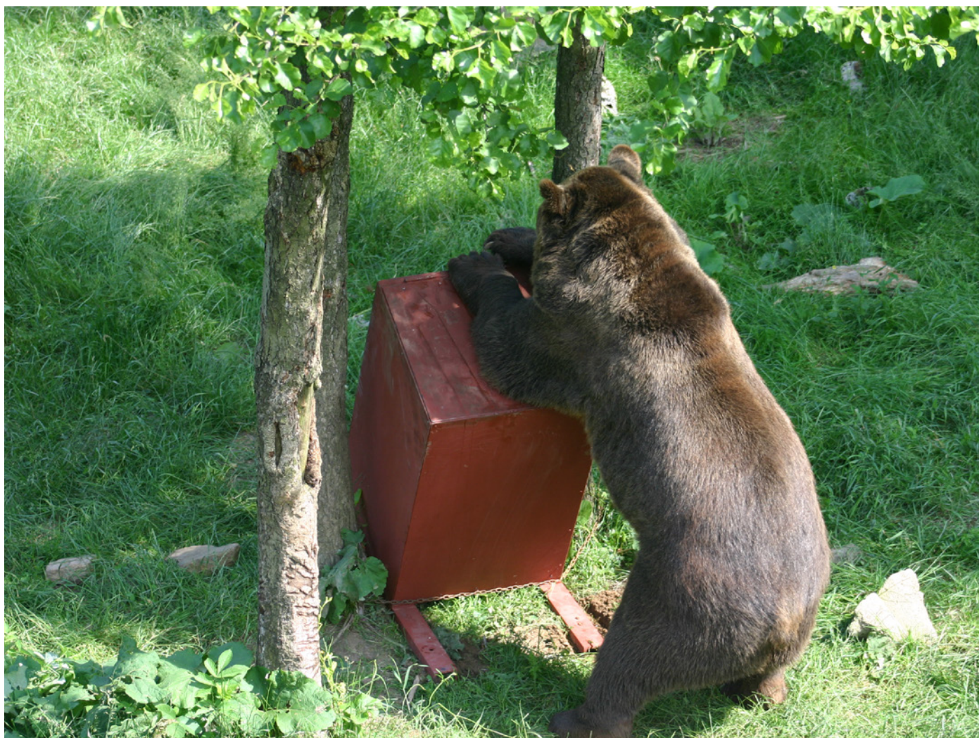
Fig. 6. Testing the efficacy of a bear-resistant refuse container (Photo: Robin Rigg).
